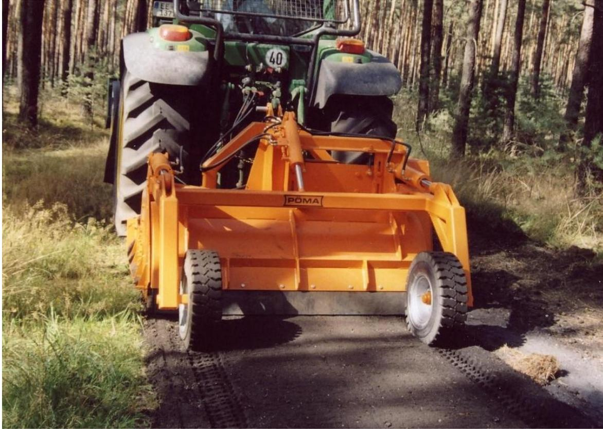
The PÖMA – Stone-crusher SB 182 is made for very heavy work. All kinds of stones can be crushed. The biggest diameter could be up to 30 cm.
